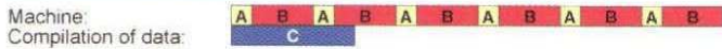
Fig. 16. Comparison of mapping methods for a 3-axis machine: (A) setup phase, (B) data acquisition phase, and (C) evaluation phase.
